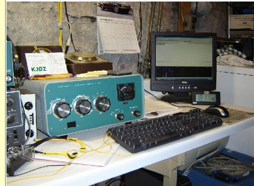
As with most shacks, this one is crowded. The keyboard and screen are separated from the Kenwood by the amplifier but there isn't much need to tune the rig anyway. All the tuning is done with the mouse and waterfall display.
