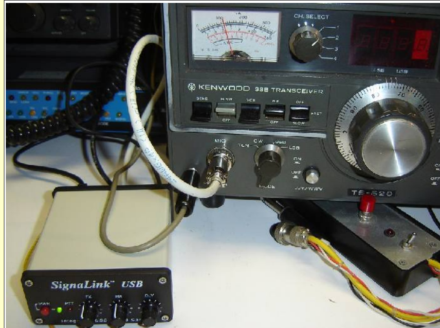
The Signalink is hooked up the the Kenwood. The white cable is from the PTT/Mic jack to the interface while the gray cable is receive audio from the earphone jack. A USB cable connects the interface to the computer USB port.
