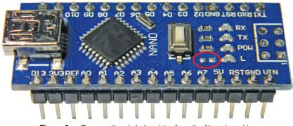
Figure 2 — Remove the circled resistor from the Nano board to disable the LED.
