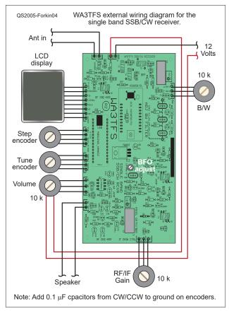
Figure 3 — The wiring external to the PCB.
