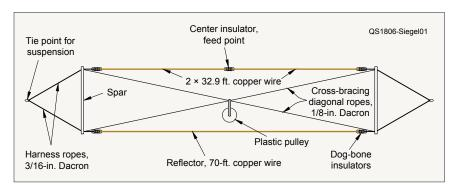
Figure 1 — Top view of the harness and the wire Yagi antenna. The RG-8X coax (not shown) connects to the center insulator and drapes over the plastic pulley. The antenna measures 95 feet between tie points.
