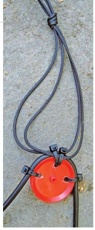
Coax cable strain relief plastic pulley assembly.
