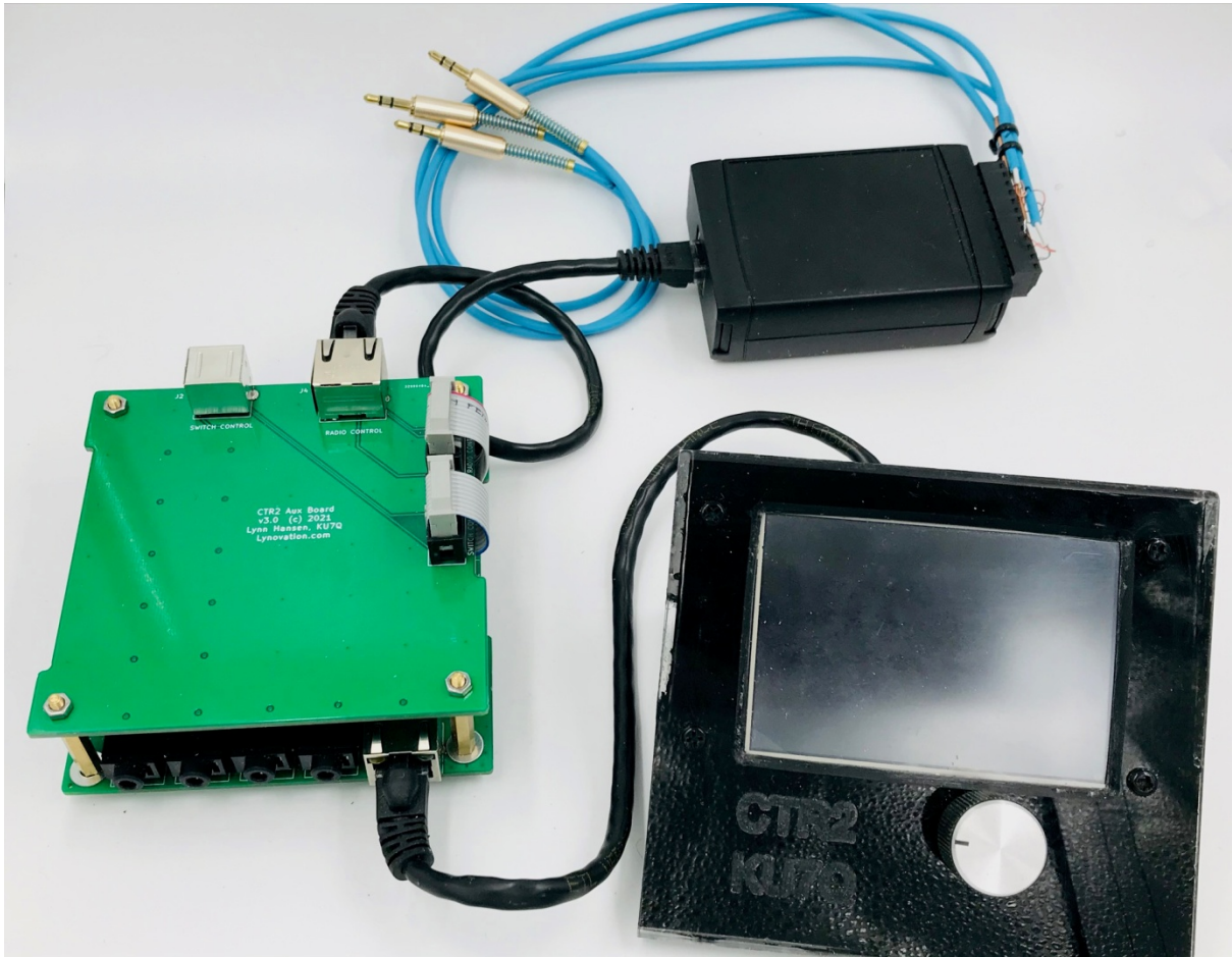
CTR2 HMI with Display, Auxiliary board, and one Radio I/O module.
