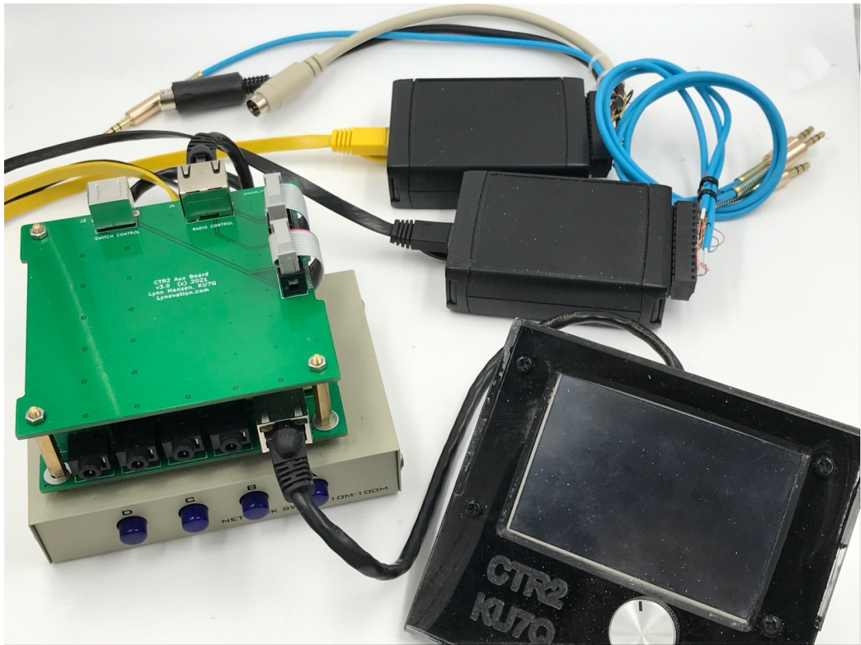
CTR2 HMI with Auxiliary board, display, manual RJ45 switch, and two Radio I/O modules.
