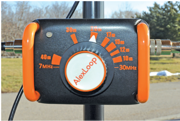
Figure 6 — The HamPack version provides a smooth gearing tuning system with a big knob and an LED SWR indicator for fast and easy adjustment of the “sweet spot.”
