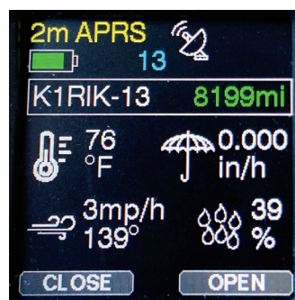
Figure 3 — Receiving weather station data via the local APRS network.
