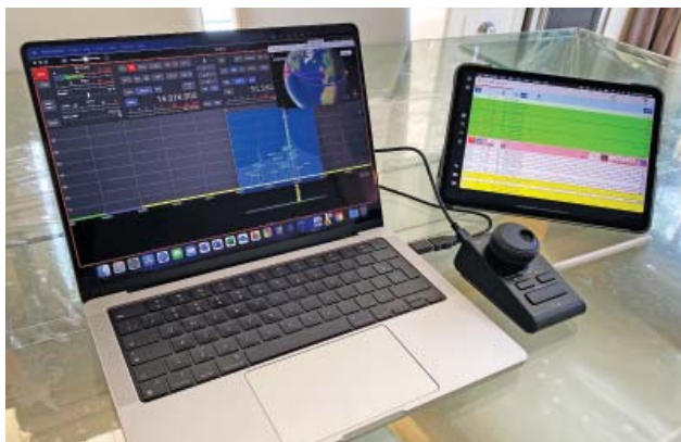
Figure 8 — The SDR-Control with the Icom RC-28 remote encoder running on a MacBook Pro, with the iPad Pro used as a secondary display (with Apple Sidecar) while in FT8.
