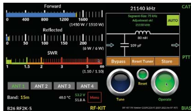
Figure 1 — A 7-inch color touchscreen is used for monitoring and controlling the RF2K-S.
