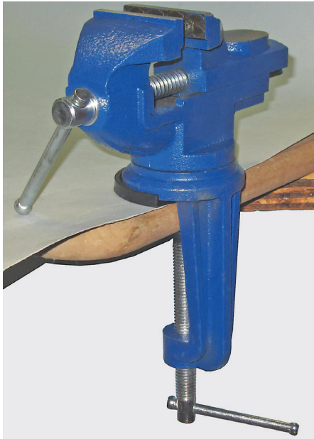
Figure 9 — Made of cast metal, the MYTEC vise includes soft jaw covers and soft inserts to prevent scratching the mounting surface or work. Without the soft inserts, the clamp mount can fit a benchtop as wide as 3½ inches.
