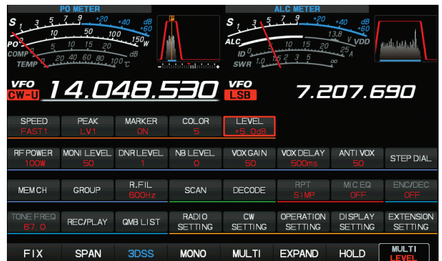
Figure 7 — Pressing the FUNC button below the screen opens up the top menu display. The MULTI button is used to select the desired function, and pressing the desired function button brings up the adjustable parameter, or an additional layer of menu items.
