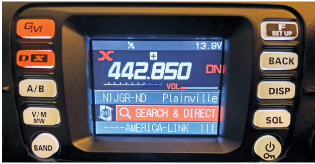
Figure 3 — Connecting to a System Fusion repeater, and then connecting to the America Link group on the Yaesu WIRES-X network.
