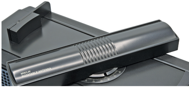
Figure 8 — The Elite 750's built-in ferrite bar antenna works well for AM broadcast band reception.
