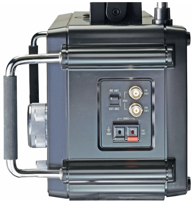
Figure 9 — The Etón Elite 750's external antenna connectors.
