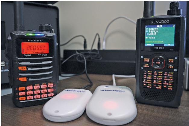
Figure 6 — The simultaneous reception of the same C4FM reflector using two different digital radios with two hotspots. On the left is a Yaesu System Fusion radio connected through an openSPOT2, and on the right is a Kenwood radio in D-STAR mode using the openSPOT3. The received signal from the reflector is transcoded from C4FM to D-STAR by the openSPOT3, and the received signal sounds the same on both radios.
