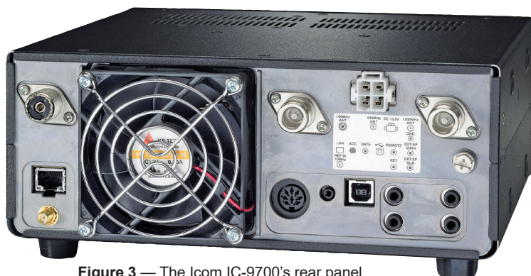
Figure 3 — The Icom IC-9700's rear panel.
