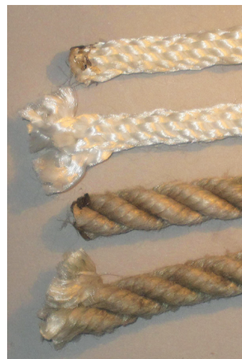
Figure 14 — The two different synthetic rope samples show how the end frays when cut with a knife. The other two ends were cut with the Weller 9400 gun and cutting tip, which melts the rope as it cuts.
