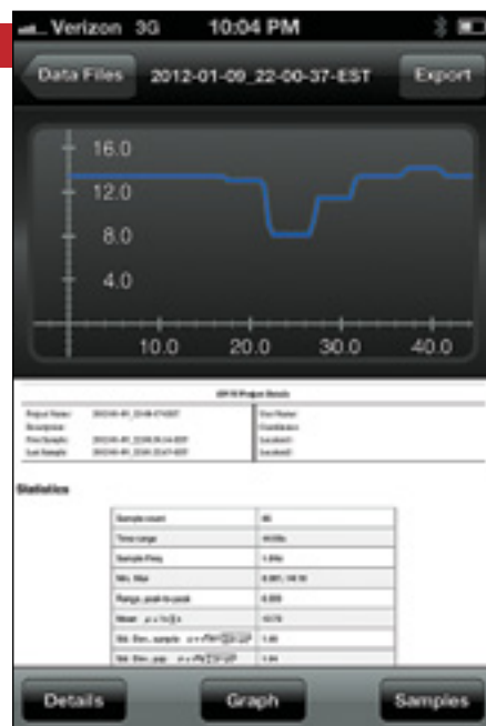
Figure 1 — The iDVM graphing function showing dc voltage variations over approximately 60 seconds.
