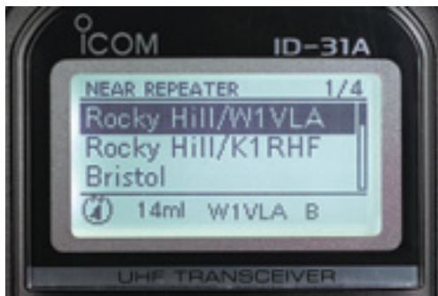
Figure 3 — Based on your position as determined by the internal GPS receiver, the ID-31A will display a list of the nearest D-STAR repeaters. Simply highlight the repeater you wish to use, select it and you're all set.
