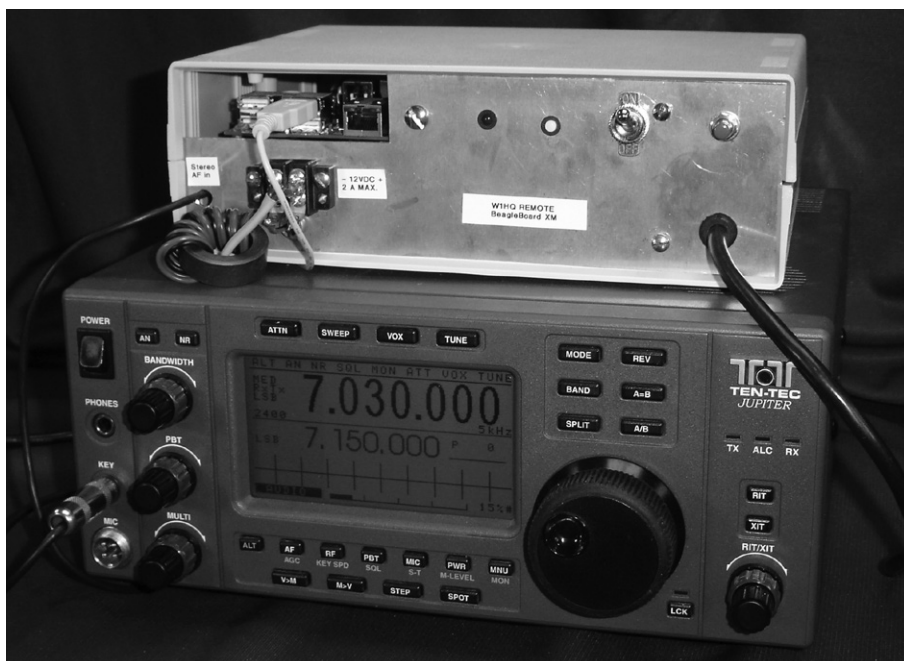
Figure 2 — Here is the remote control box containing the BeagleBoard XM computer and the Ten Tec Jupiter transceiver.
