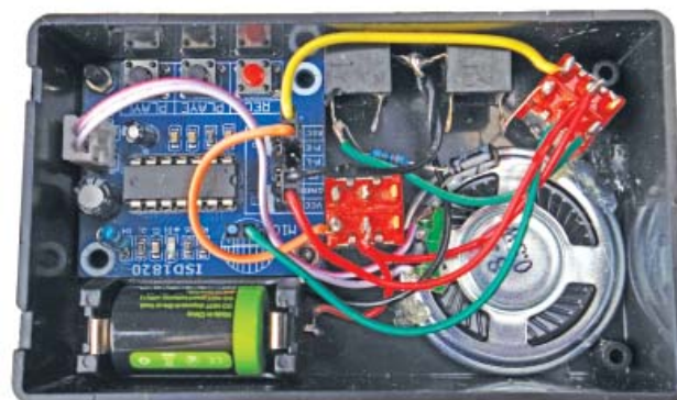
Figure 1 — An internal view of the voice keyer. The ISD1820 module is on the upper left, and the battery is on the lower left.
