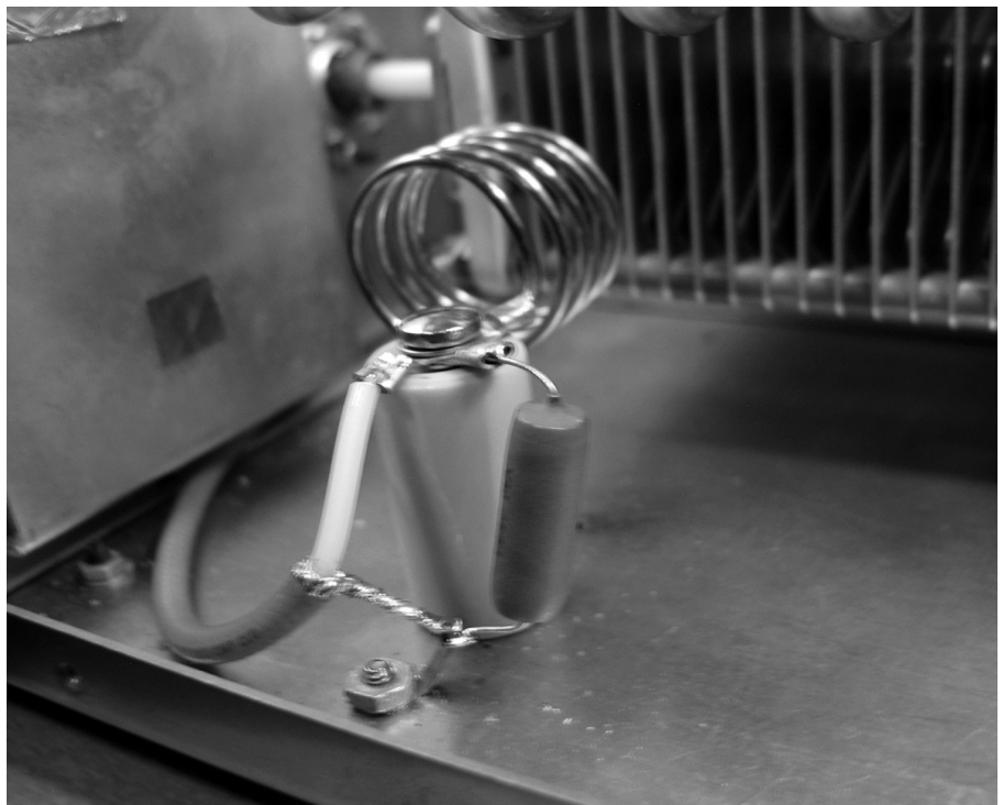
Figure 3 — Inductor L2 mounts on a ceramic stand-off and connects to the RF output coax (below and left) and to choke RFC1. The other end of RFC1, and the coax shield connect to the ground lug at the bottom.
