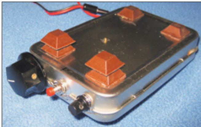
Figure 9 — Rubber stick on pads are used to elevate the front of the case about 1 inch and the rear about ½ inch.
