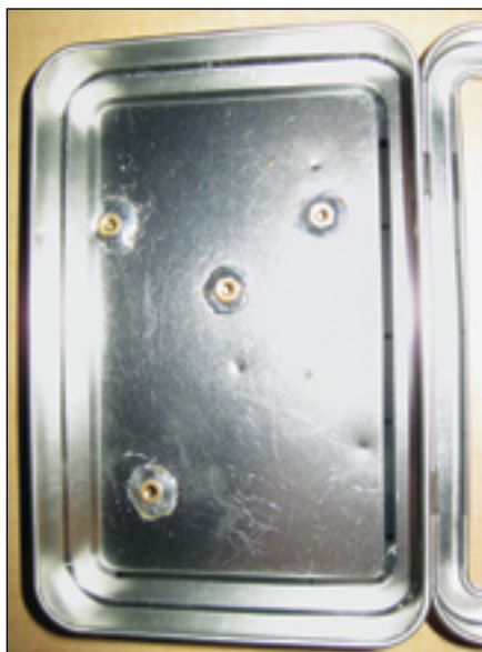
Figure 8 — Case with the mounting nuts soldered in place.
