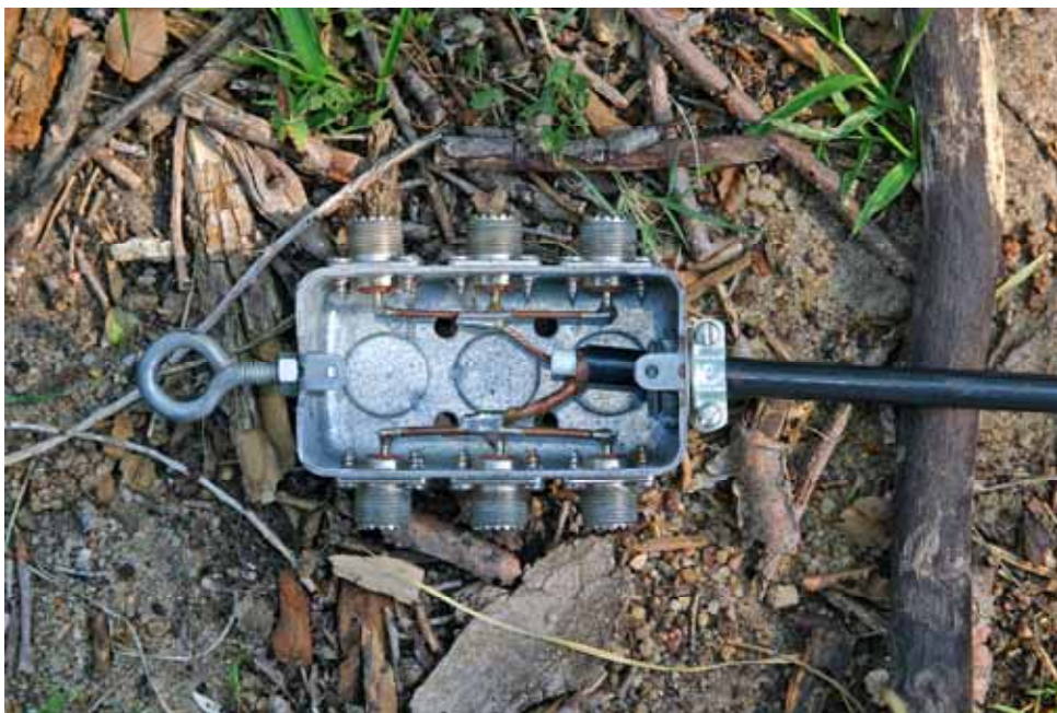
A NØLRA-designed dipole box is easy to make out of common parts.
