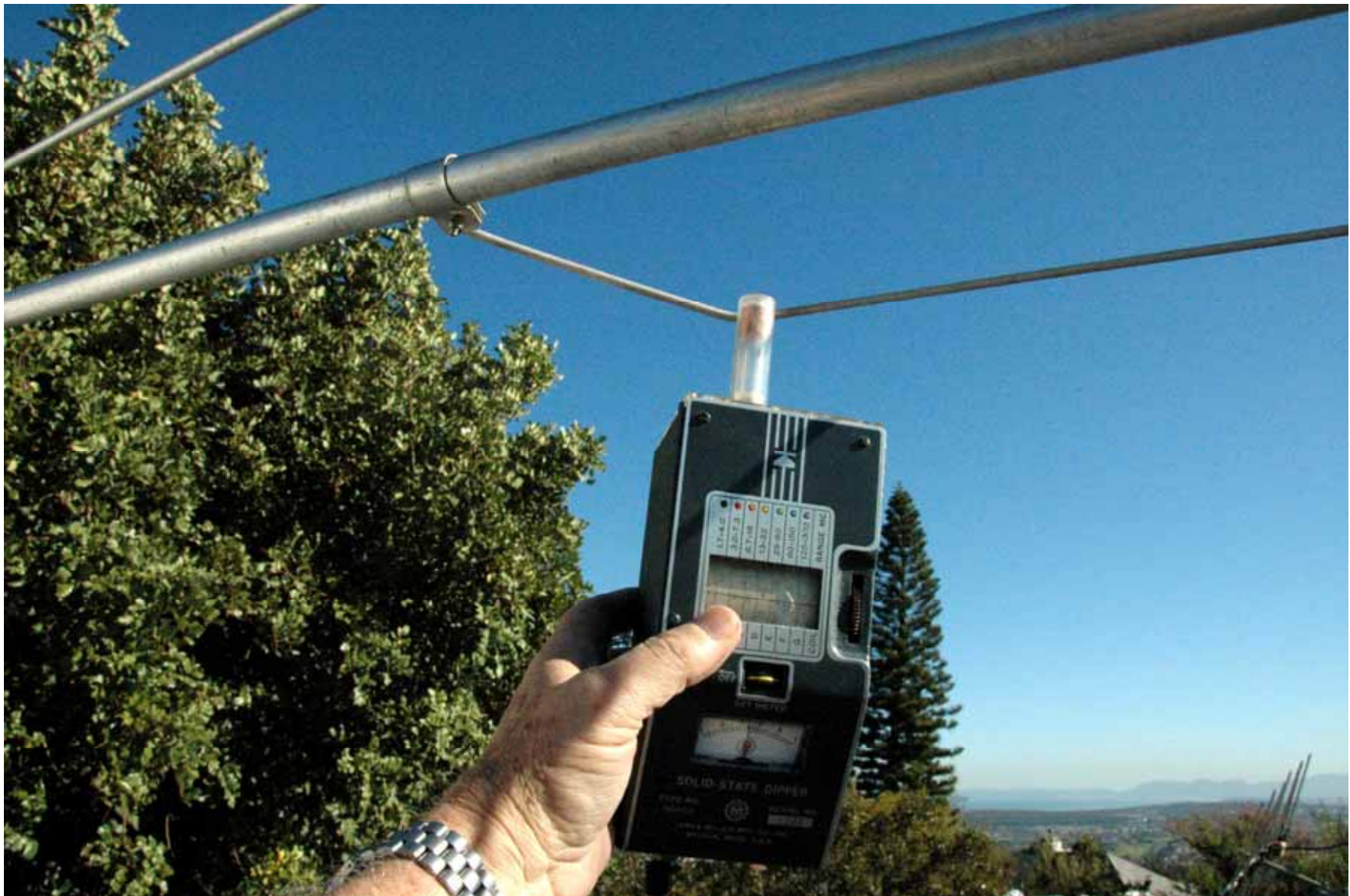
Figure 11 — Bringing the linear resonator to resonance at 22.5 MHz using a dip meter.
