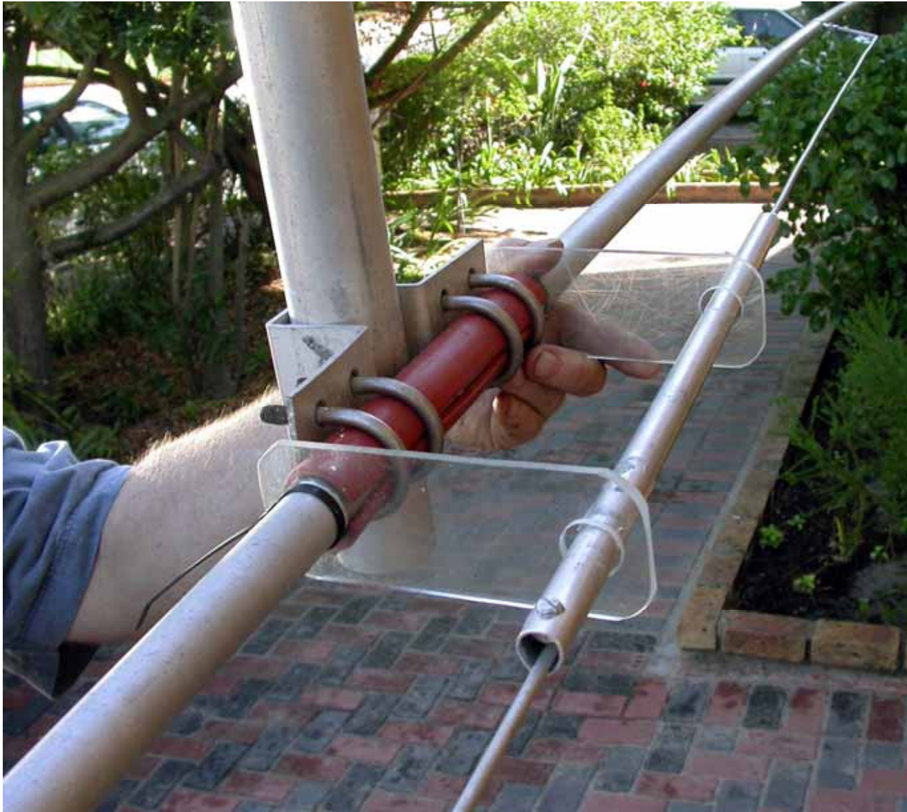
Figure 4 — A completed linear resonator attached to the 20 meter reflector. In this view the boom is pointing up.
