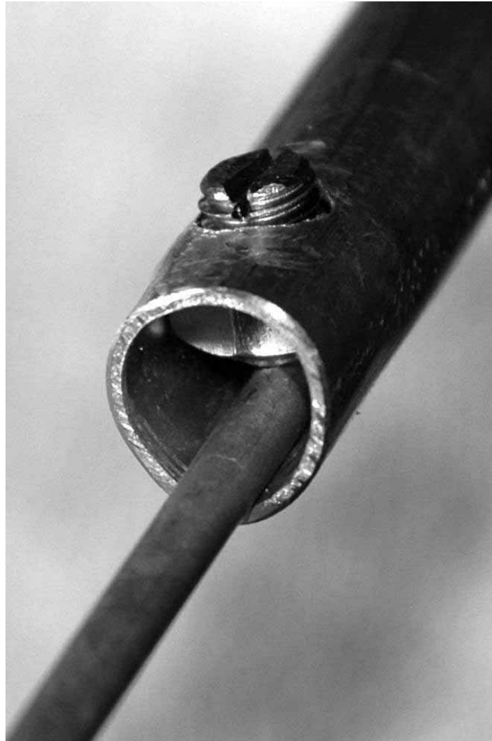
Figure 7 — A close-up view of the nut and lock screw (part M) in the end of the tube (part B) where they are used to secure the rod (part A).
