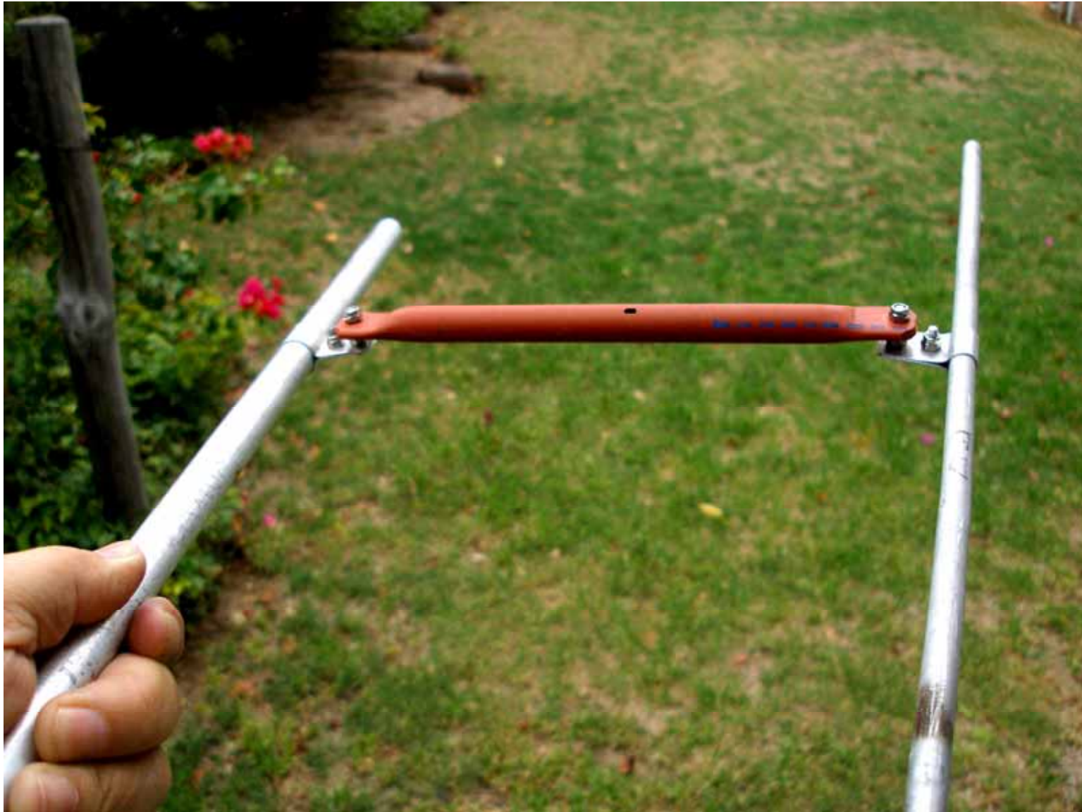
Figure 12 — Photo of the mounting method for the 12 meter dipole.
