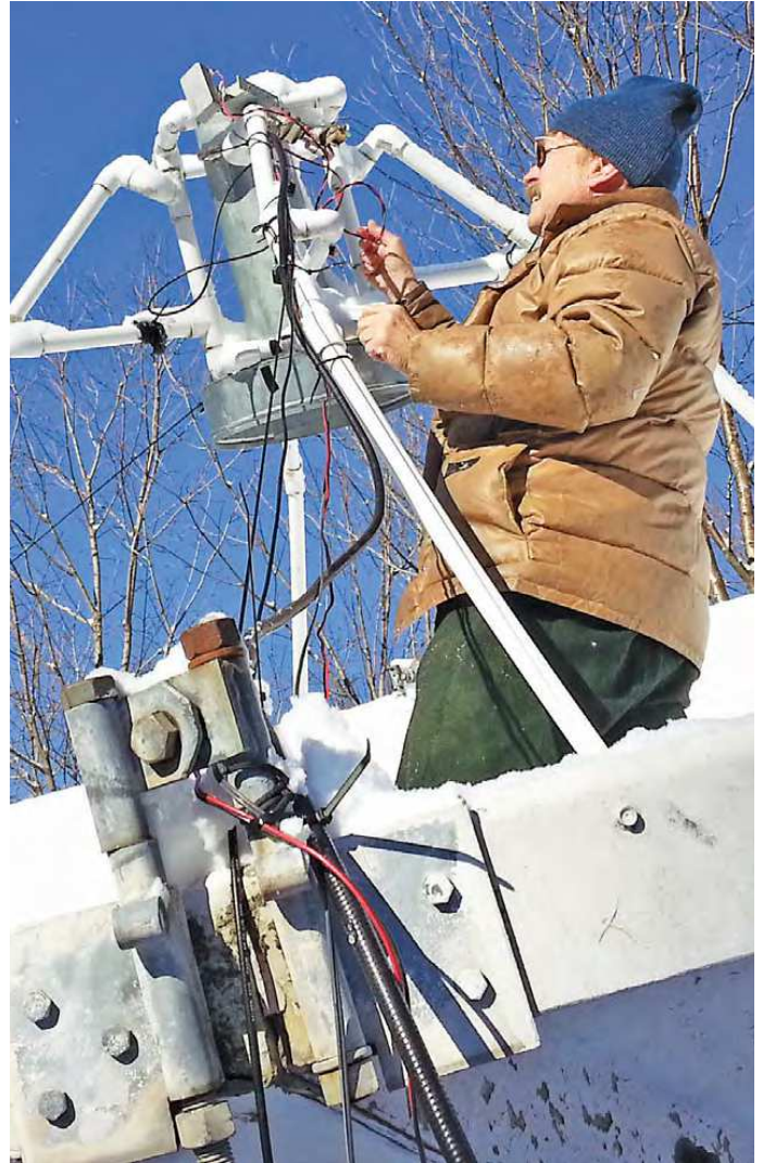
Figure 3 — Larger feed horns for lower frequency bands can be fabricated from sheet metal, like the one Chip Taylor, W1AIM, is adjusting on his 16-foot dish for 1296 MHz.
