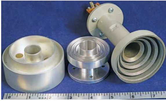
Figure 2 — Choke rings improve dish gain and efficiency to make better feed horns. On the left are single and multiple choke rings for prime-focus. At the right is a conical horn with rings for an offset feed horn.
