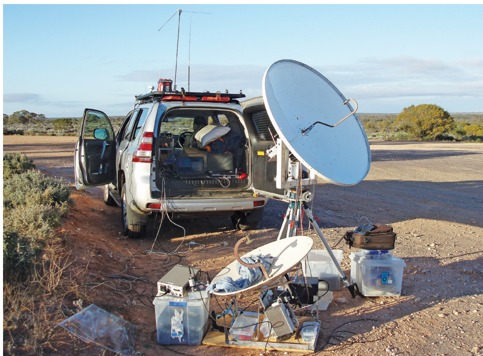
Figure 3 — VK7MO operating small-dish EME in the Australian outback. The 24 GHz station is on the tripod and the 10 GHz rig on the ground. [Rex Moncur, VK7MO, photo]
