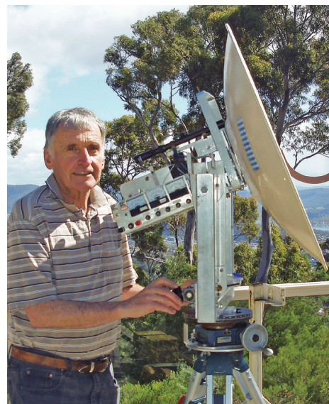
Figure 2 — Rex Moncur, VK7MO, conducting a 10 GHz small-dish EME experiment with a 77-centimeter dish. [Noel Foley, photo]
