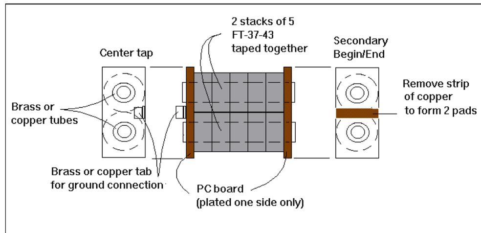
flashing copper to form the center tap. Be sure to leave a tab on the center tap for connecting to the circuit board. Make two similar tabs for the secondary connections on the other end of the cores. Wind three complete turns through both cores with Teflon insulated AWG #22 stranded wire. The wire ends should extend out of the core end with the center tapped secondary.
