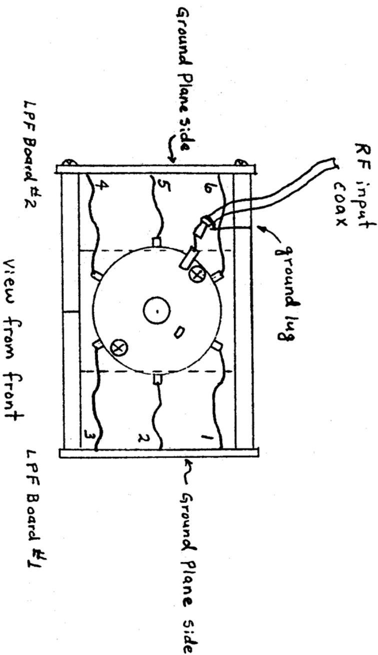
Figure 5, Low Pass Filter Assembly Details
