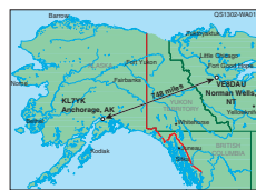
Figure 1—This 6 meter contact between K179K and CPEP spanned 748 miles using only 80 W and an attic loop.
