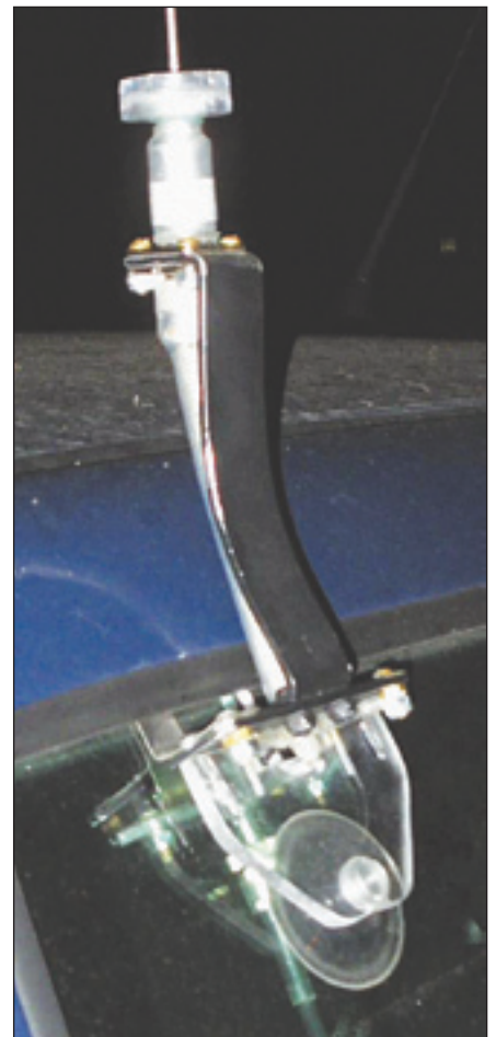
Figure 6 — Side view photo of completed mount installed on window.
