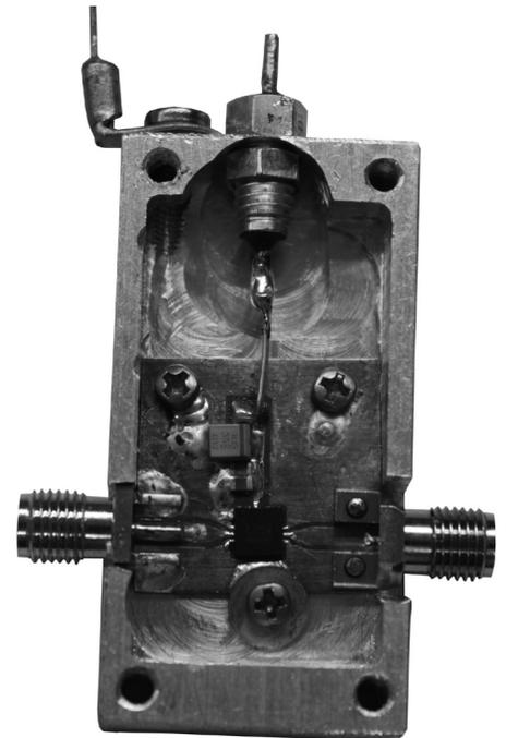
Figure 11 — Assembled multiplier/doubler in a machined aluminum housing.
