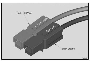
the 30-A Anderson PowerPole connector. Not only can the PowerPole handle greater current, it is also capable of being plugged and unplugged many hundreds of times (operations) without deterioration. These connectors are available from several *QST* advertisers including Cable X-Perts (www.cablexperts.com) and PowerWerx (www.powerwerx.com). More information is available from the Anderson Power Products Web site at www.andersonpower.com. Look for these part numbers:
