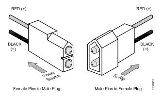
The 12-A Molex 1545 series connector (part numbers: male, 03-09-2022; female, 03-09-1022) is adequate for low power mobile radios, handhelds and accessories.
