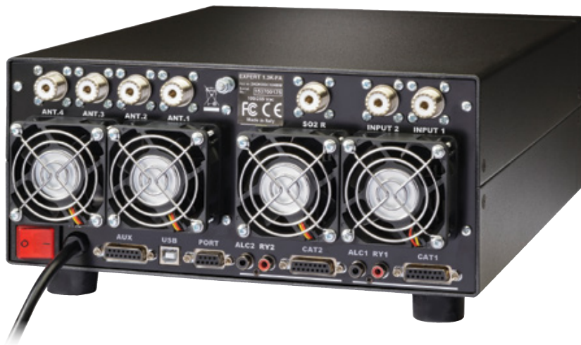
Figure 9 — Rear-panel view of the SPE Expert 1.3K-FA amplifier. The four antenna connectors are at the upper left, while the RF input for two radios and the SO2R connector are at the upper right. Along the bottom are connectors for interfacing two transceivers and USB and serial ports for computer connectivity/remote control.
