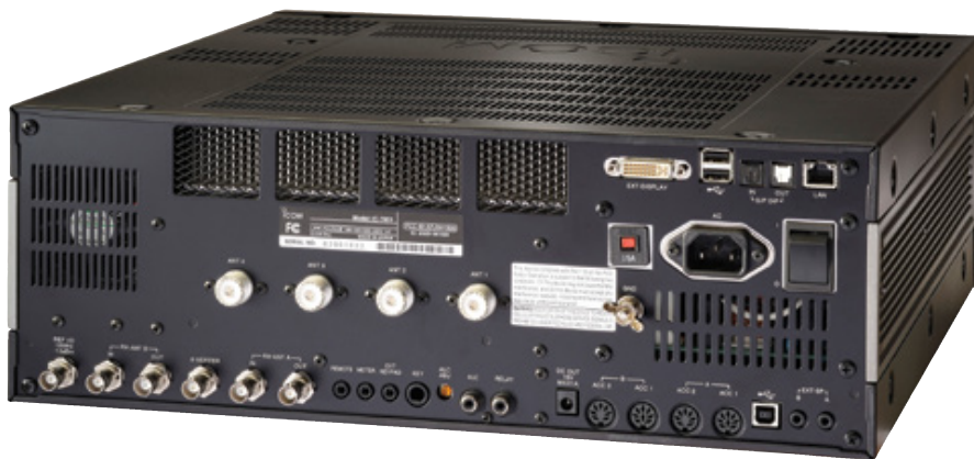
Figure 1 — The rear-panel view of the IC-7851. While there are many connectors for various functions, normal operation can be conducted with just the 120 V ac power cable, one or more antenna connections, and a ground connection. When you want to do something requiring additional flexibility, the other options will likely be appreciated.
