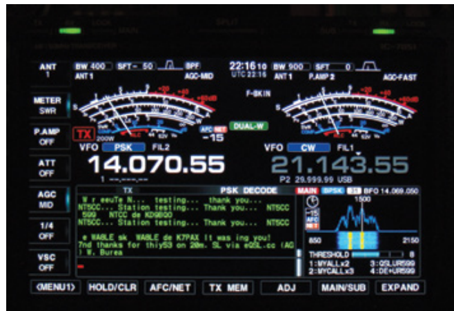
Figure 8 — Similar to Figure 7, but in PSK mode. The main differences are the additional PSK phase-indicating circle and the single center frequency. Each mode has its own set of recorded transmit messages.
