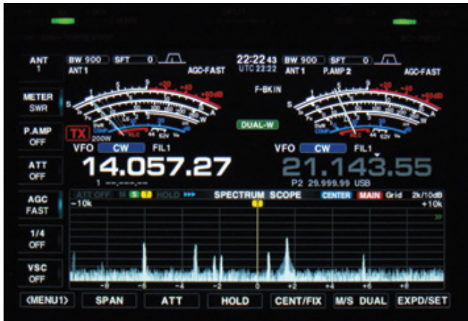
Figure 2 — A view of the front panel display of the IC-7851 during CW operation. Note that both receivers are active on different bands and the spectrum display is showing \pm 10 kHz around the operating frequency of the main receiver. Note particularly the S meters — they are digital images that look just like real moving-coil D'Arsonval meter movements.
