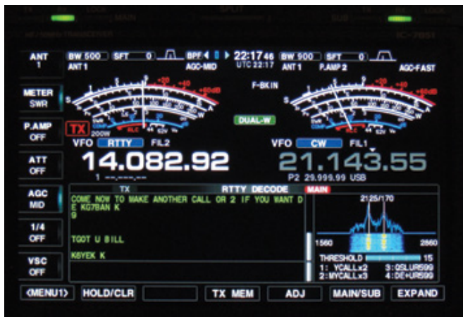
Figure 7 — The display during RTTY operation. Note the window on the lower right that provides tuning information by comparing the received spectrum to the RTTY mark and space frequencies. On the lower left is a screen portion with up to eight lines of decoded receive text. Below that is a space for a type-ahead buffer ready to send upon shift to transmit mode. Below the mini spectrum and waterfall displays are summaries of the first four transmit memories to allow sending via a keypad or connected keyboard. The transmit memories in detail can also be displayed on the lower portion of the screen to allow transmission via soft buttons, if the keypad or keyboard is not available.
