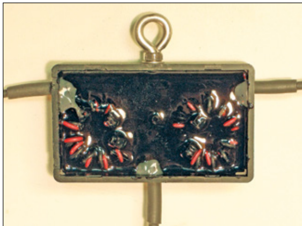
Figure 7 — The 3.3-inch-wide Aerial 51 Model 404-UL matching unit with the cover removed. The antenna wire and coax connect within the sealed unit. The hang-up eye is the way to support the antenna.
