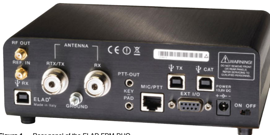
Figure 1 — Rear panel of the ELAD FDM-DUO.
