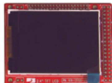
Figure 6 — The larger (4½ × 2½ inch) PC board contains the microprocessor, controls, and analog front end parts. The smaller board (2¾ × 2 inches) holds the 2.4-inch TFT LCD screen.
