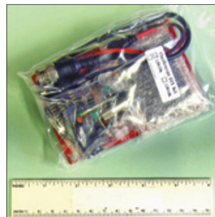
Figure 7 — It's hard to believe that this small bag of parts (including the probe) is all you need to make a fully functional oscilloscope.
