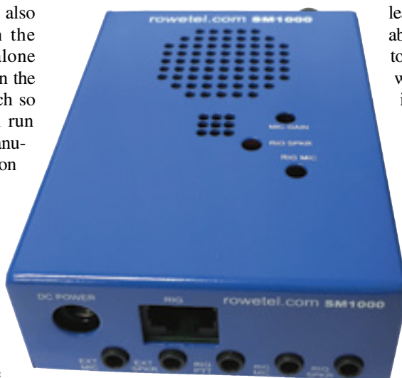
Figure 5 — The SM1000 can connect to the transceiver via the RJ45 RIG connector, or the individual 1/8-inch phone jacks along the bottom of the case.
