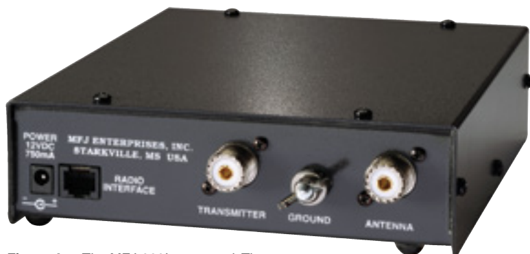
Figure 4 — The MFJ-939I rear panel. The separate POWER jack is not used when a transceiver interface cable is connected.
