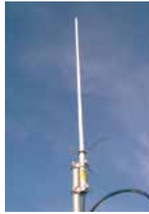
Figure 3: You can also use a roof- or ground-mounted antenna, such as this Comet GP-3, with your handheld.
