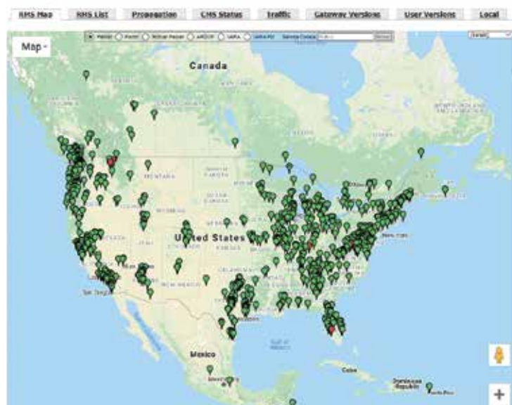
Figure 2: A map of all Winlink Remote Message Server (RMS) stations within the US, Canada, and Central America that can be accessed by VHF packet radio.
