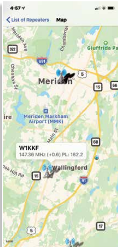
Figure 2 — A repeater map screen from the RFinder smartphone app. Notice that the W1KKF repeater is using a 162.2 Hz CTCSS tone, although here the tone frequency is labeled “PL.”
