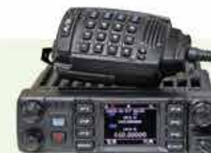
The AnyTone AT-D578UV is a dual-band FM and DMR mobile transceiver.
