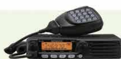
The Kenwood TM-281A is an example of a single-band (2 meters only, in this model) FM-only transceiver.
