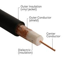
Coaxial cable is made of two conductors, one inside the other. In this example, the outer conductor (or shield) is made of braided copper wire. It completely surrounds the center conductor, which in this cable is made of stranded copper wire. The insulating dielectric in this example is made of white plastic. The exterior of coaxial cable is covered by a plastic jacket.
