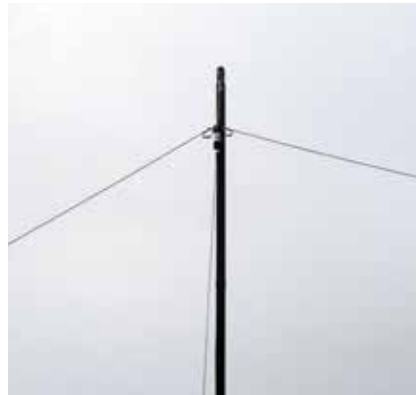
Figure 4: This wire dipole antenna is attached to a single support and the wires slope downward like an upside-down V. This is known as an inverted V configuration.
