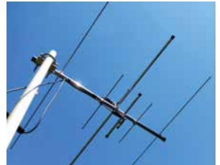
Figure 3: A Yagi antenna like this VHF/UHF model will focus your power in a particular direction.
