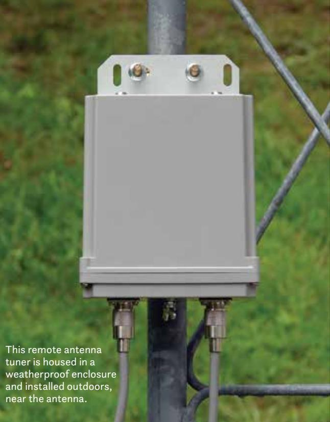
A grey, rectangular remote antenna tuner is mounted on a metal pole. The tuner has a weatherproof enclosure with two mounting holes at the top. Two coaxial cables are connected to the bottom of the tuner. The background is a blurred green field.
