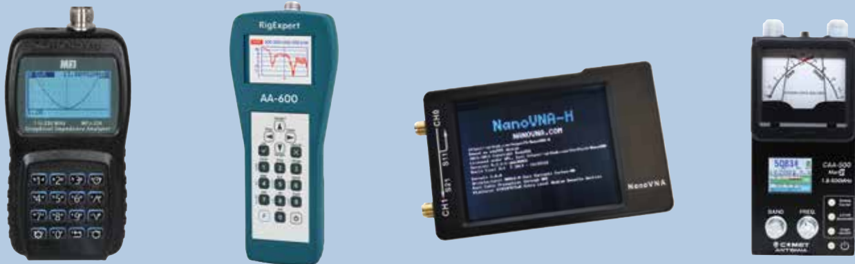
Above, left to right: An MFJ analyzer doing a frequency sweep to find the lowest SWR. ■ A RigExpert AA-600 analyzer doing an SWR sweep through a broad range of frequencies. ■ The NanoVNA sells for less than $100. ■ The Comet CAA-500 Mark II analyzer offers a mechanical meter and a graphic display.
