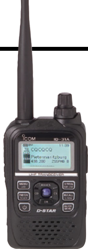
The ICOM ID-31A is a dual-band D-STAR handheld that also receives and transmits analog FM.
