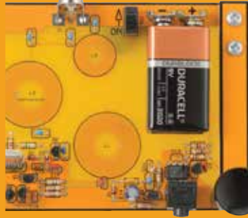
Modern CW transmitters can be very simple, such as this battery-operated Cricket transmitter available from the 4 State QRP Group at 4sqrp.com .
