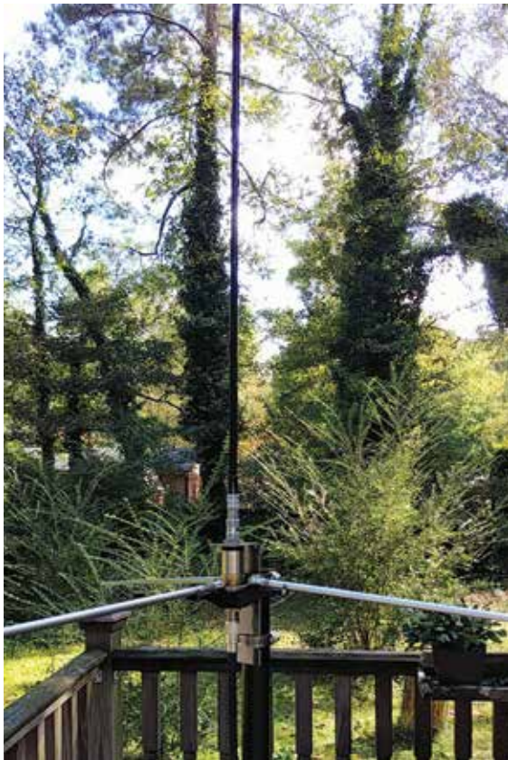
The finished project includes a ground plane with radial rods that help complete the antenna circuit.
