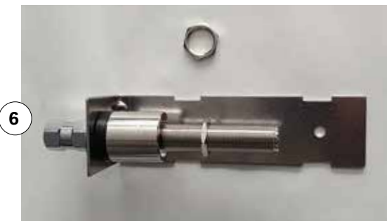
Screw the bulkhead connector into the bottom of the Diamond adapter. Apply your wrench to the lower of the two nuts and use it to tighten the connector into place.
