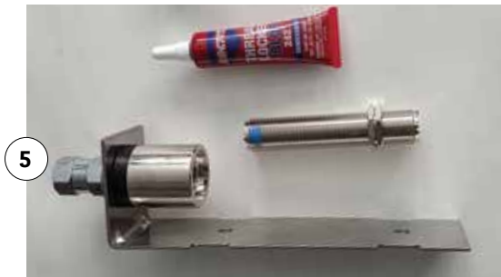
Thread two nuts onto the bottom of the 4-inch bulkhead connector. Place the nuts so that they touch each other. Add a drop of thread lock to the threads at the opposite end of the bulkhead connector.
