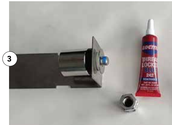
Insert the Diamond 3/8 x 24 adapter and the bottom and top washers. Add a drop of thread lock to the adapter threads at the top.
