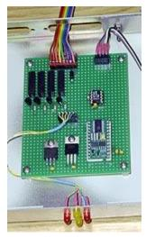
I suggest the interface be constructed and tested in stages. Begin first by wiring and testing the voltage regulators. Next add the BASIC Stamp and serial port. The BASIC Stamp is
