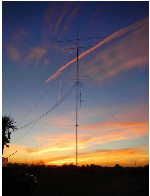
Hector, XE2K, used this 8-element Loop-Fed Array on 6 meters. (Photo by XE2K)
