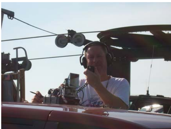
Rich, NØHJZ, making a 270 km contact with 2 watts and a 17 dB horn antenna. (Photo courtesy NØHJZ)
