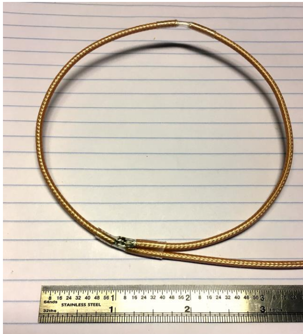
Figure 7. Completed pickup loop, about 3 inches diameter.
