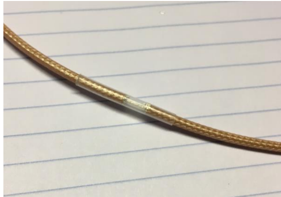
Figure 5. Midpoint gap in the shield is covered with heatshrink.
