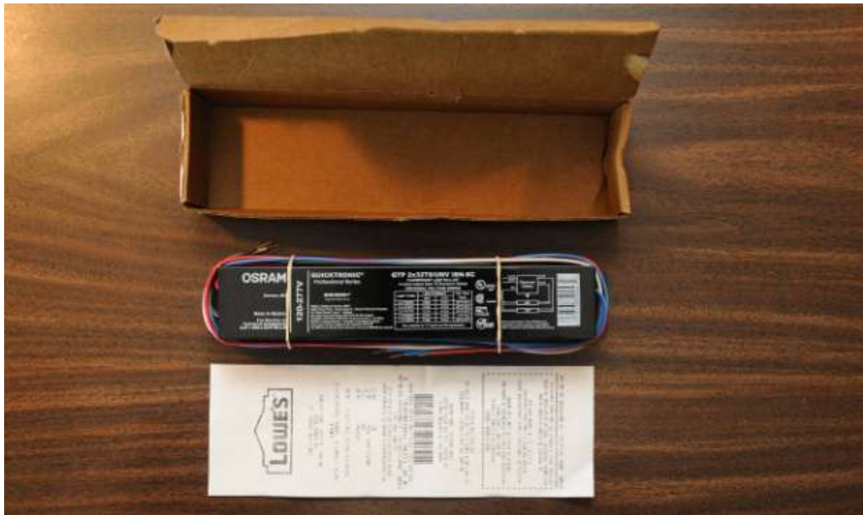
Figure 3.4 – Inside the box. FCC rule § 18.213 (d) requires manufacturers of RF lighting devices to include an advisory statement on product packaging or in documentation. This statement describes and addresses the device potential to cause radio interference. Although small print on the ballast indicates, “Complies with FCC 47 CFR Part 18, Non-Consumer No PCBs,” the required advisory statement was not included on the product packaging. There was no documentation included with the device in the box. This is a labelling violation on the part of the manufacturer.
