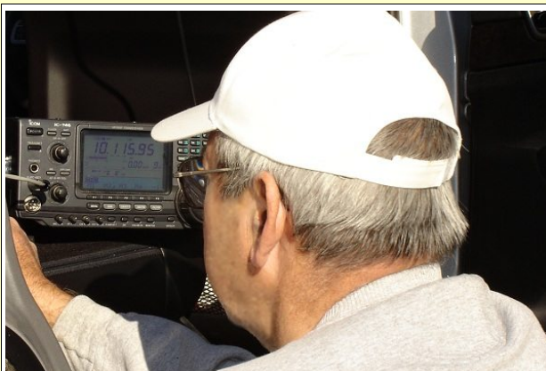
The ICOM 746 is powered up and the auto tuner has matched the antenna to the radio. I've placed the CW key on the seat next to the radio in a comfortable spot
