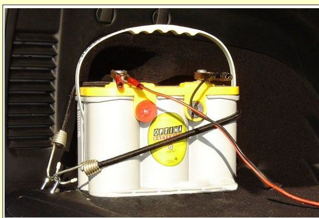
The Optima battery is held in place with bungee cords. A special power cable with alligator clips connects power from the radio to the battery
