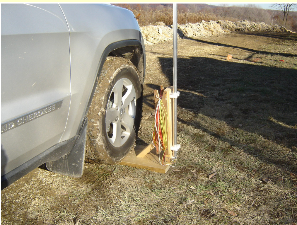
The Jeep has been driven onto the base of the antenna support. The SO-239 RF connector is visible at the base of the aluminum mast
