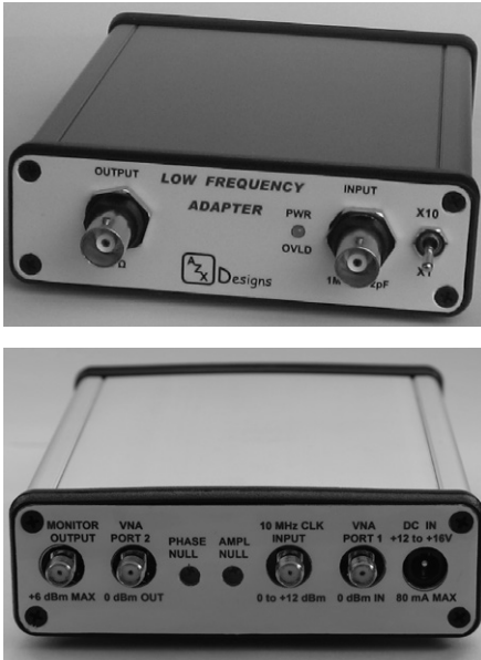
Figure 6 — The low frequency adapter is built in a standard Hammond extruded aluminum cabinet. The front and rear panels are pictured.
