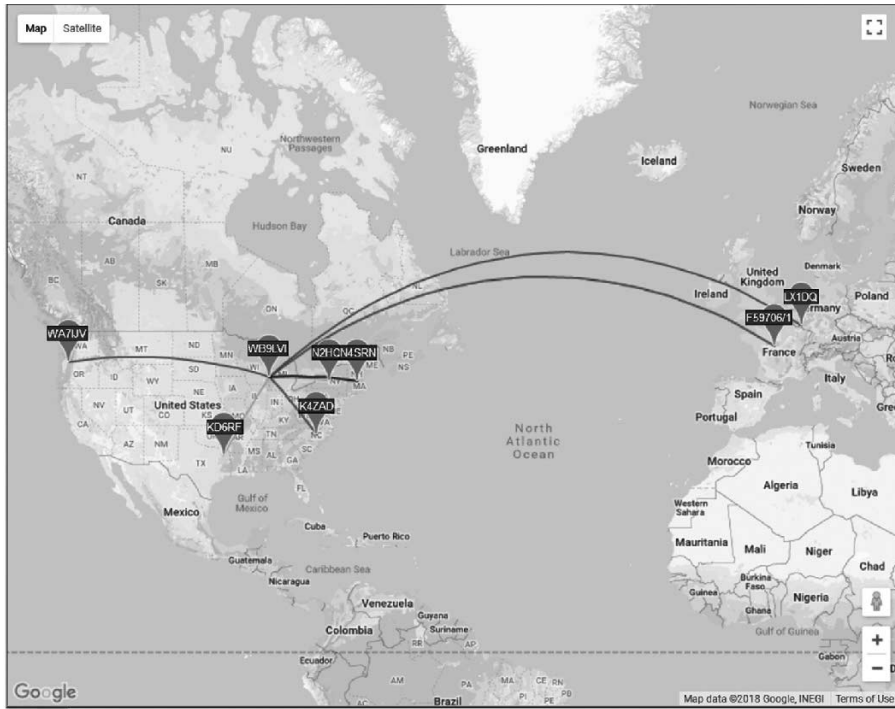
Figure 2 — Photo of WSPR map showing receptions of this unusual transmitter on the 17 meter band.
