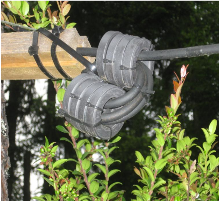
Figure 10. On the left, the choke installed an electrical half-wave from the feed point of the 80 meter prototype. The pieces of wood shown in the photograph are to prevent chafing of the coax by tree bark. On the right, the choke installed at the feed point of the 40 meter prototype. A choke is necessary to prevent current from flowing on the coax braid, which prevents the antenna from achieving its predicted excellent SWR across the whole band.
