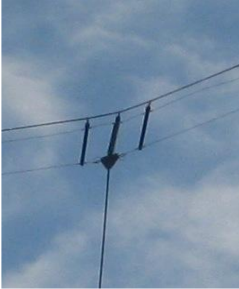
Figure 6. Center spacer, flanked by two others, as described in the text. A commercial center insulator hangs from the center spacer.
