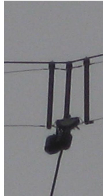
Figure 10. On the left, the choke installed an electrical half-wave from the feed point of the 80 meter prototype. The pieces of wood shown in the photograph are to prevent chafing of the coax by tree bark. On the right, the choke installed at the feed point of the 40 meter prototype. A choke is necessary to prevent current from flowing on the coax braid, which prevents the antenna from achieving its predicted excellent SWR across the whole band.
