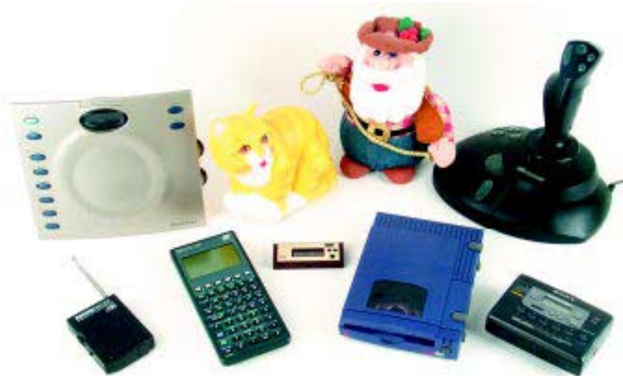
Part 15 devices are everywhere. This collection was scavenged from an Editor's work area. Part 15 covers most any electronic device that keeps time or interacts with the user in any way. In this group, the cat meows when there is movement nearby and the stuffed cowboy sings a digitally recorded Christmas tune.
