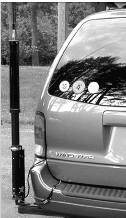
The High Sierra HS-1800 is a so-called “screwdriver” style HF mobile antenna that provides continuous coverage for all HF bands.
